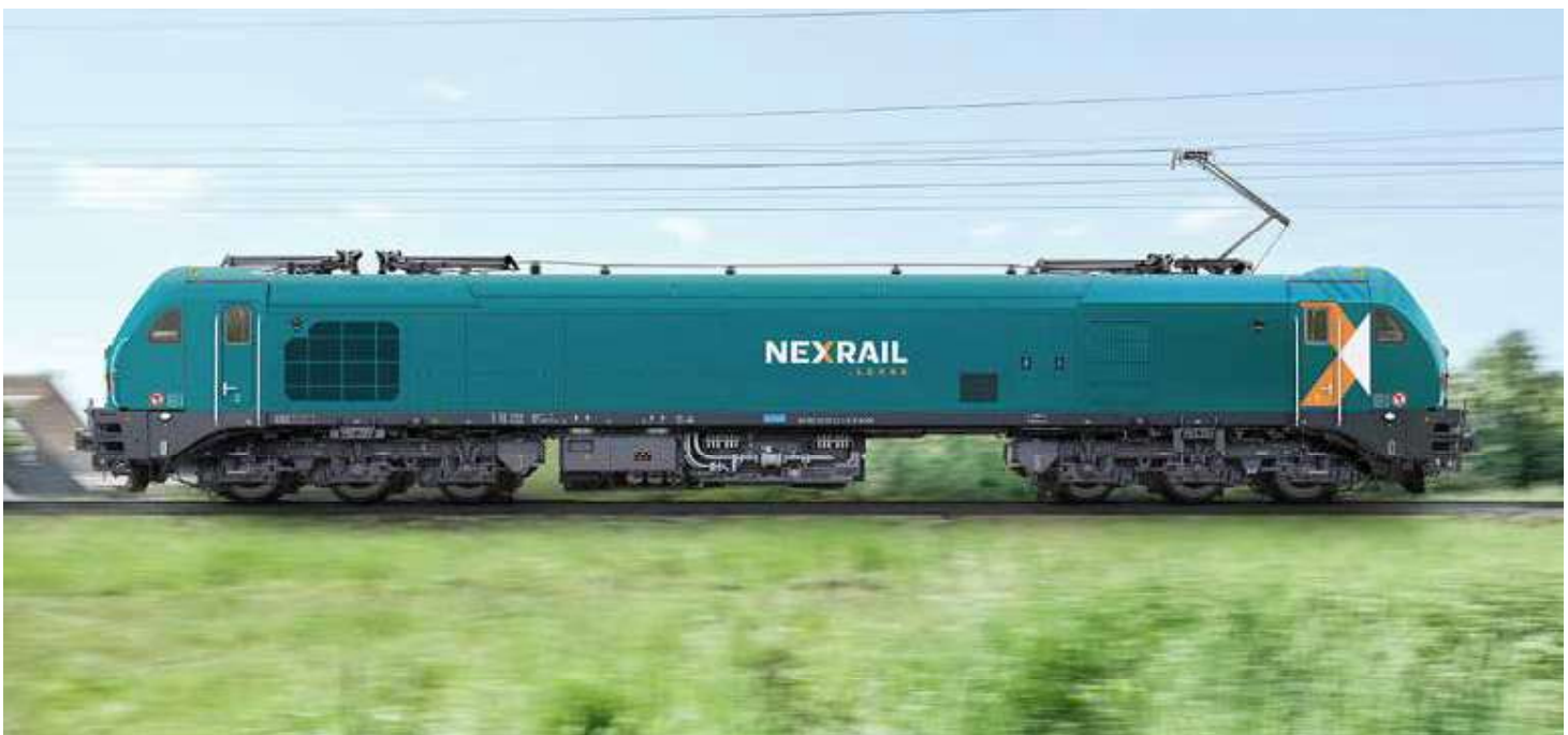
✘ The EURO9000 panto-battery hybrid locomotive.
