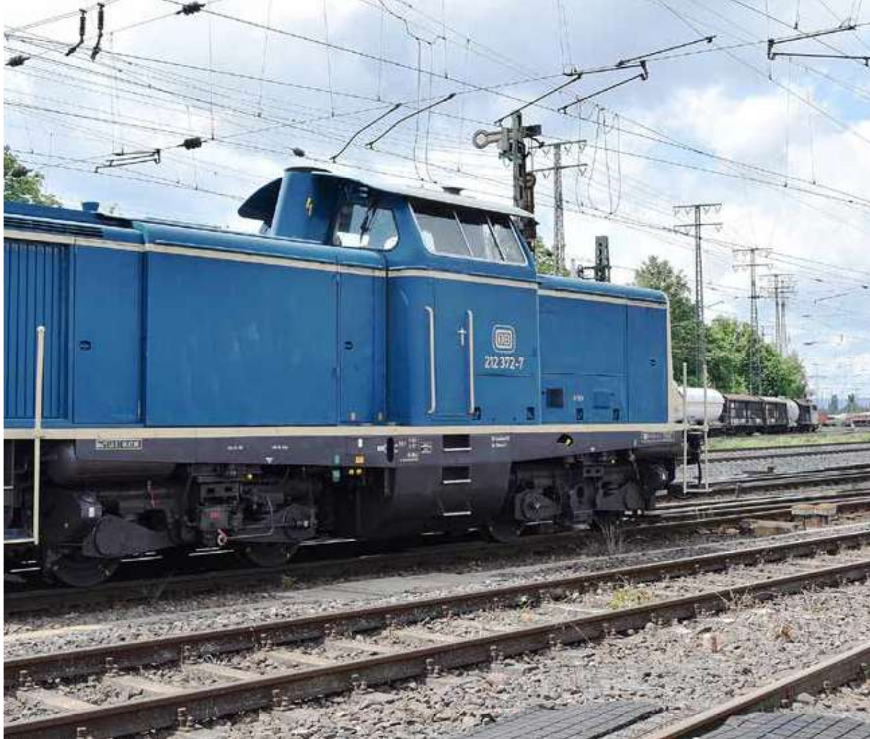
✘ An old V100 diesel-hydraulic locomotive in use with Deutsche Bahn.
